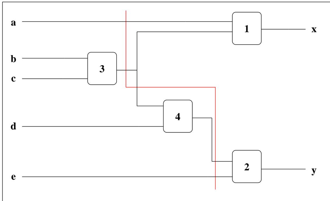
At any time, the \*BMD expresses the word-level representation of the output as a function of the nets currently crossed by the cut.
