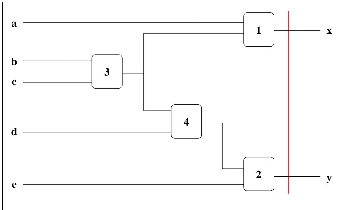
**Beginning of the algorithm:** the cut crosses all the primary outputs. The \*BMD of the word-level interpretation of the output is constructed.
