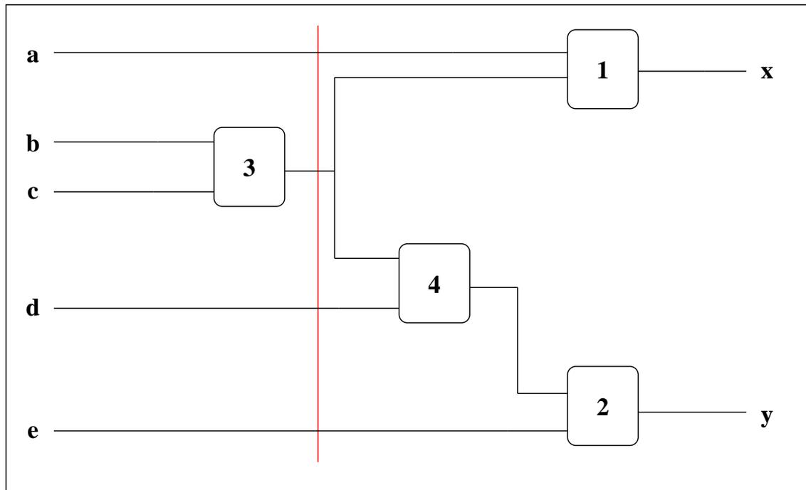
**Condition:** a gate may be chosen only if its output is connected to only the input of the gates that have been already taken.
