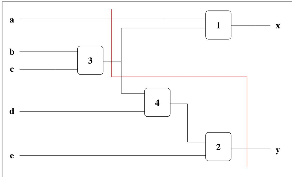
A gate just left to the cut is chosen and its output is substituted in the \*BMD by the corresponding function of its inputs.
