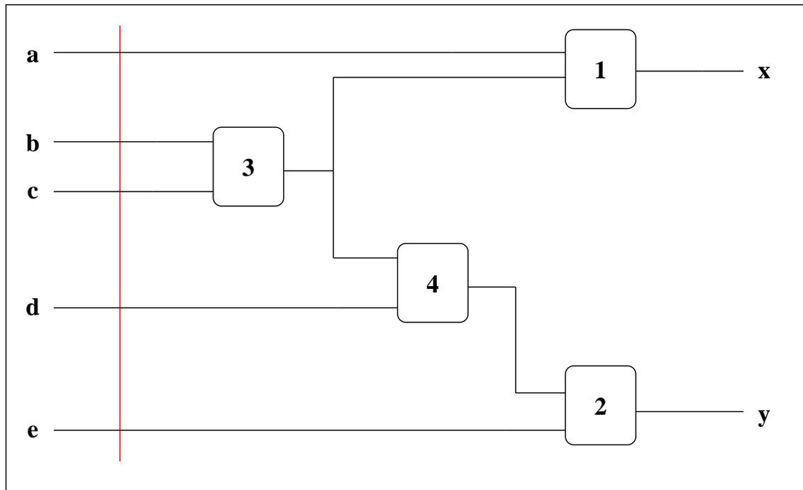
**End of the algorithm:** the cut crosses all primary outputs. The \*BMD expresses the word-level representation of the output as a function of the inputs.
